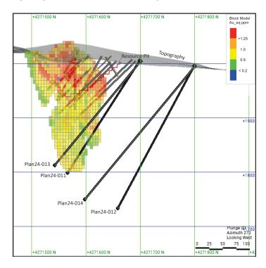
Section through proposed drill holes at the Calvada East target. Proposed drill holes are shown in black, previous drill holes with gold grade are also illustrated. Note that the conceptual pit (shown in red) which constrains the project's MRE does not capture the deeper resource blocks. Successful drilling will extend mineralization deeper, and potentially, the conceptual pit shell as well.
