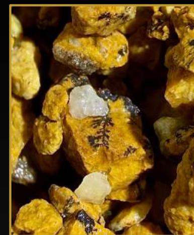
RC cuttings with MnO x dendrites: high grade Ag, up to 648 g/t Ag
