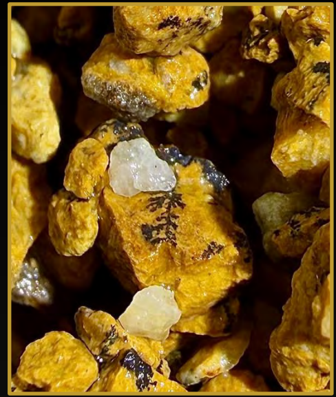
RC cuttings with MnO x dendrites: high grade Ag, up to 648 g/t Ag
